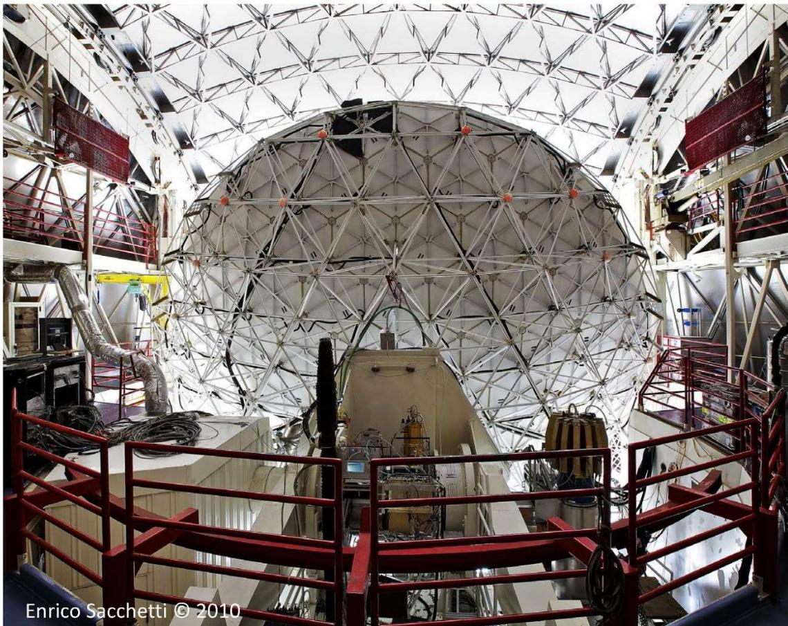
Figure 1-4: Panoramic, interior view of the CSO and telescope with the author's receiver (2010). This spectacular photo from the CSO mezzanine was taken by photographer Enrico Sacchetti (© October, 2010) [14]. It shows the receiver cryostat mounted on the telescope's Cassegrain Relay Optics assembly situated between its two elevation axis bearings [9].
