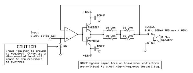
The 4x68 Ohm resistors give a total of 1W power dissipation, which is required.
